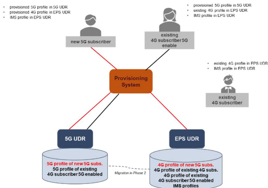
Figure 3. Storage of subscriber data through provisioning system
