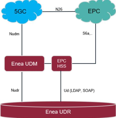
Figure 4. UDM with basic EPC HSS functionality
