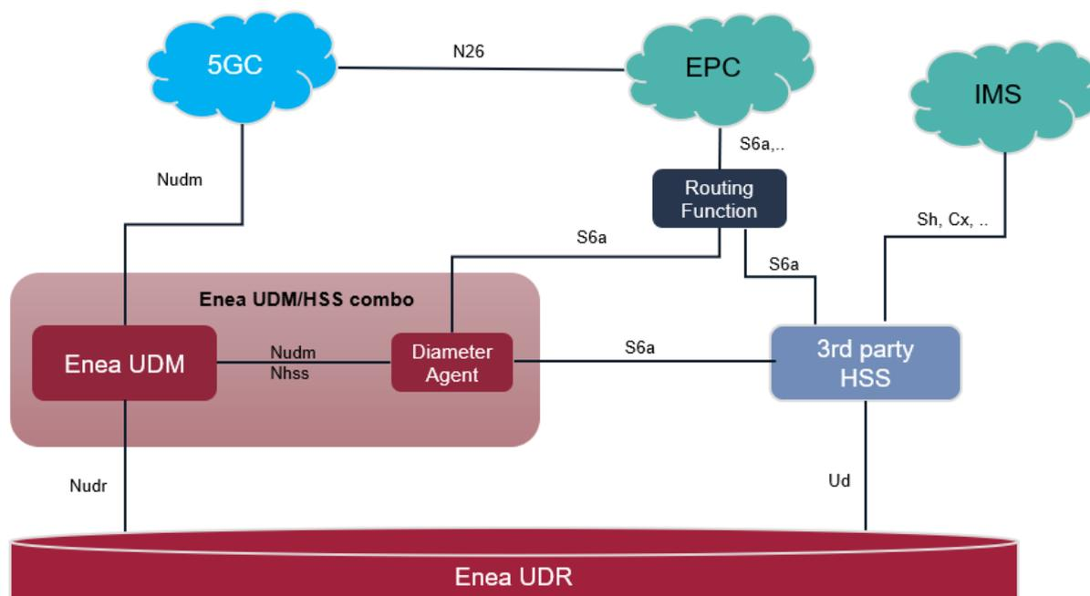
Figure 2. Interworking as UDM/HSS Diameter interact
