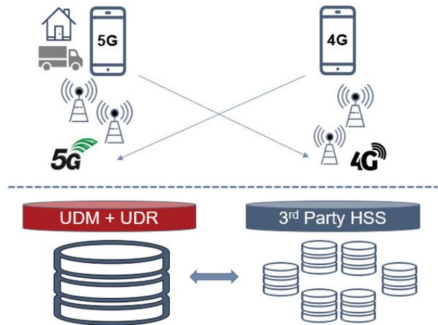
Figure 5. Separate repositories for 4G and 5G interacted with use of a Data Access Layer for between HSS FE and the UDM.
