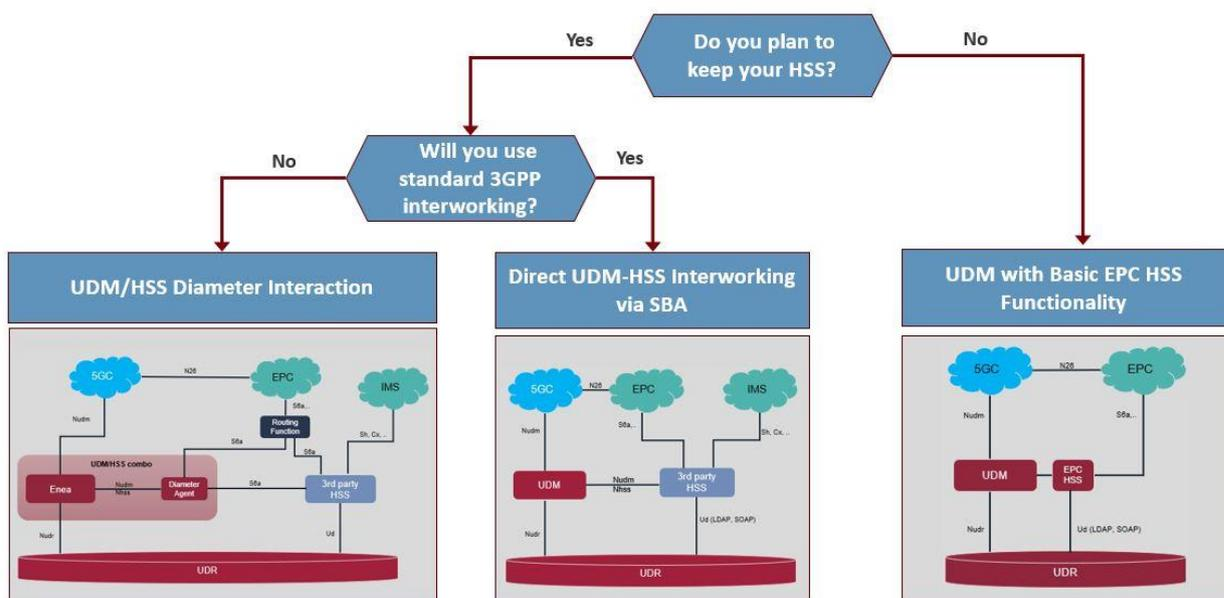
Figure 6. Data management architectures resulting from decisions made between the interworking options
