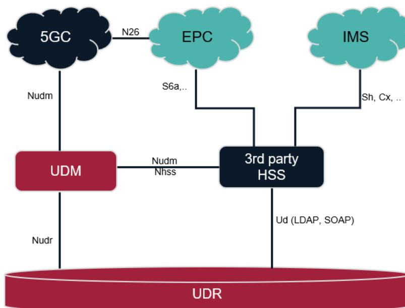
Figure 1. Interworking with SBA, the UDM supports Nudm and Nhss for 4G interworking with 3rd party HSS
