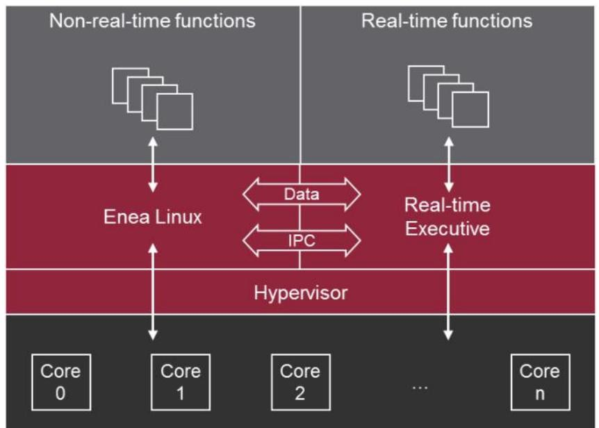
Overview of the dual OS partitioning approach to enable real-time in Linux on multicore devices
