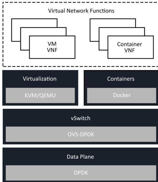
Figure 2. Enea NFV Access configurations.
