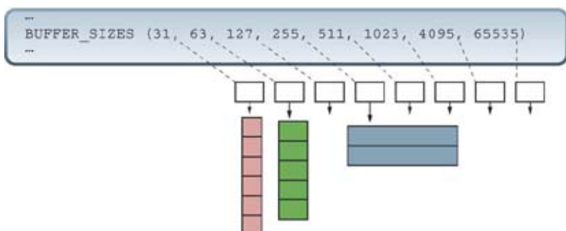
Figure 10. Enea OSE Memory Pool Buffer Reuse via Free Lists.
