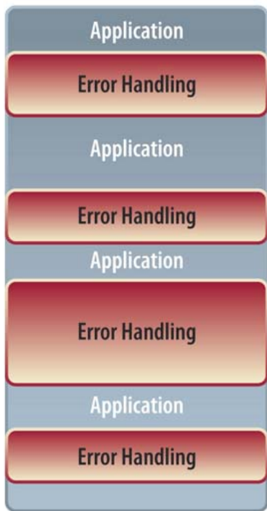
Figure 13. Enea OSE Error Escalation Sequence.
